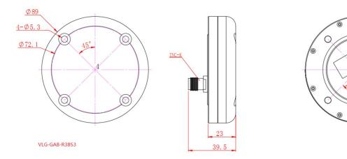
**Installation:** Antenna equipped with 4 through hold  $\phi$ 5.3, user can fix the antenna through these holes by
